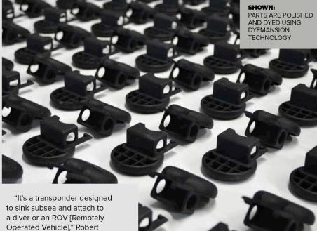
"It's a transponder designed to sink subsea and attach to a diver or an ROV [Remotely Operated Vehicle]," Robert Kovacs, Senior Subsea Design Engineer at Kongsberg Maritime tells TCT. "It is used when you want to know precisely where it is located in relation to other subsea instrumentation on a work site."
